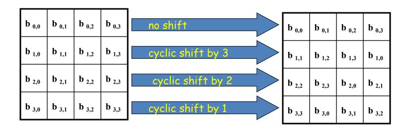
ShiftRow operates on the rows of the State. The purpose is to provide inter column diffusion.
