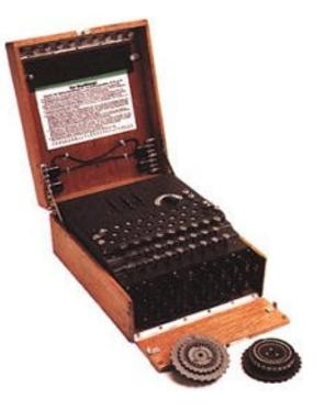
At least once a day the Germans changed the order of the rotors, their starting positions and the plugboard connections. To decipher a message sent using Enigma, you had to work out exactly how all of these had been set.
